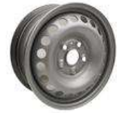
FT92841 JANTE D'ACIER GRIS 6.5J X 16" | ET52 | 5 X 120 CH65
